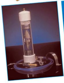
For ice makers, drinking water, cooking water and any purpose when water needs improvement of taste, color or odor. The 69 cublc inches of activated carbon will completely remove all chlorine from 1842 gallons of water when the chlorine and chloramine concentration level is .5 ppm. The activated carbon still removes a large percentage of chlorine and
