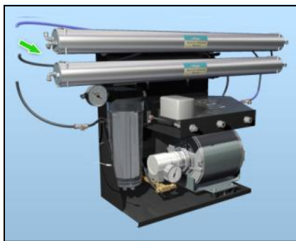
Figure 19: a) disconnect the tubing from both the RO Modules b) Remove the RO Modules from the clamps holding them to the frame You will need to install the new RO Modules in the same
