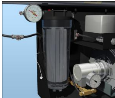
Figure 14. Move red needle to the back side of the black needle
